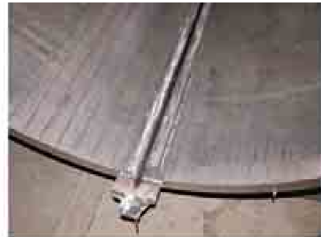
Alloy 22 Inside seam weld
