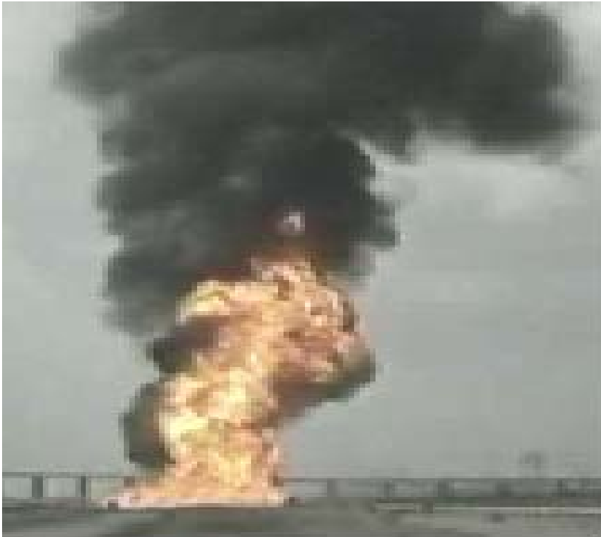
35 m dia LNG pool fire test on insulated concrete (Fire in methane burning period at ~100s after ignition)
