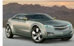
Chevrolet Volt Extended Range EV 40-mile EV range 16kWh Li-Ion Intro: 2010 CY
